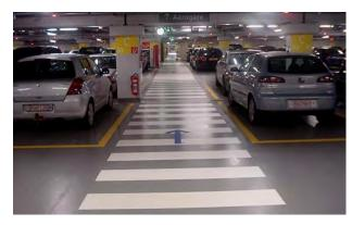
The intermediate decks of a car park are likely to have the lowest level of thermal movement, thermal shock and UV radiation. Therefore these aspects must be considered but it may, for example, be possible to use a more rigid (non crackbridging), lower thickness, lower cost resin system; dependent of course on the other selection criteria, particularly the position and condition of joints and any cracks in the decks.
